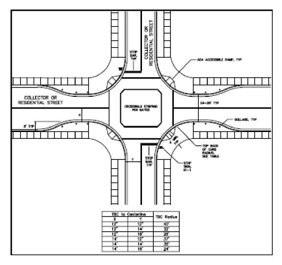
The typical *neckdown* is used in connection with on-street parking and, unlike a conventional intersection with a large curb return radius, offers a short crossing distance and high visibility for pedestrians. In the typical design, the curb return radii and street widths are such that single unit trucks can stay to the right of the centerlines when making right turns.
