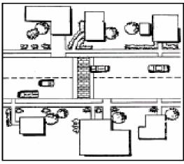
*Speed tables* are flat-topped speed humps often constructed with a brick or other textured materials on the flat section. They are also called *trapezoidal humps*, *plateaus*, and if marked for pedestrian crossing, *raised crossings* or *raised crosswalks*.
