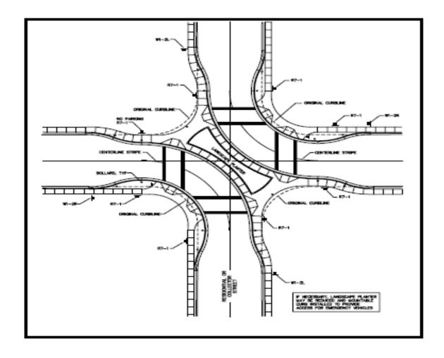
*Diagonal diverters* will have clear widths sufficient for single-unit trucks (or buses if a transit route) to make turns at treated intersections without encroaching into opposing lanes. They will have openings five to six feet, sufficient for bicyclists to pass through barriers, but not for motorists to do so.
