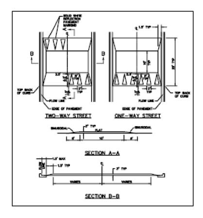
The typical *speed table* is three inches high and 22 feet long in the direction of travel. The plateau (flat top) is 10 feet long and each ramp is six feet long. The plateau is made of asphalt, concrete, stamped asphalt or concrete, or other patterned materials as approved by the Engineer.
