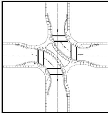
Diagonal diverters are barriers placed diagonally across an intersection blocking through movement. They are also called full diverters and diagonal road closures.
