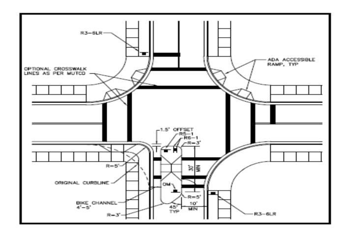
The typical *half closure* has two geometric features designed to encourage compliance with the one-way restriction. First, the curb extension or edge island extends more than a car length along the roadway. Second, the curb extension or edge island extends all the way to the centerline of the street or beyond on a wide street.
