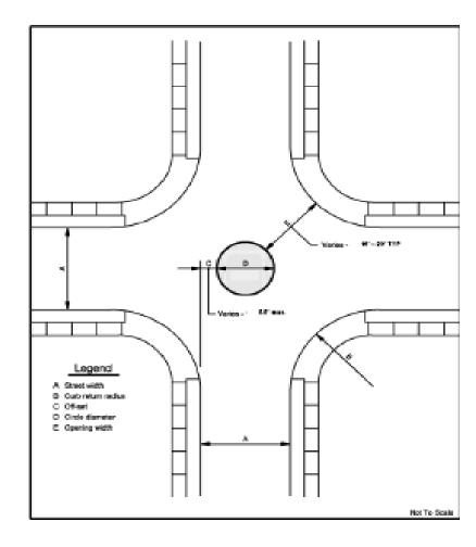
Most *traffic circles* have circular center islands and circular perimeters formed by the intersection corners. Where intersecting streets differ significantly in width, the center island may be elongated to better fit the intersection. An elongated circle consists of half-circles with tangent sections between them. Most traffic circles are deployed at four-way intersections, for this is where the greatest safety benefits accrue.
