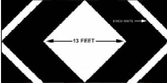
*Speed humps* are rounded raised areas placed across the road. They are also referred to as *undulations*. The standard or Watts profile hump, developed and tested by Britain's Transport and Road Research Laboratory, is the most common speed control measure in the United States (U.S.). It is the only speed control measure, at present, for which ITE provides design and application guidance.
