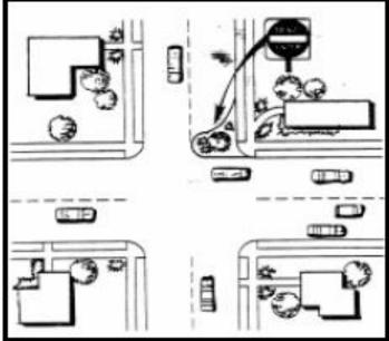
Half street closures are barriers that block travel in one direction for a short distance on otherwise two-way streets. They are also sometimes called *partial closures* or *one-way closures*. When two half closures are placed across form one another at an intersection, the result is a *semi-diverter* that blocks through movement on a cross street.
