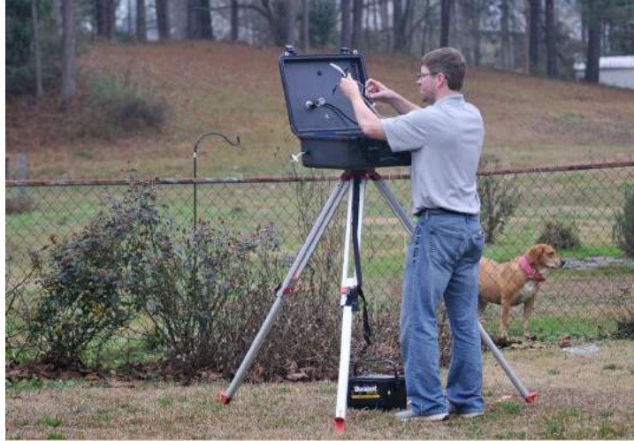
Justin Rhodes, an industrial hygienist with GHD, installs an air monitoring station in the yard of a home in Clemson Terrace.
